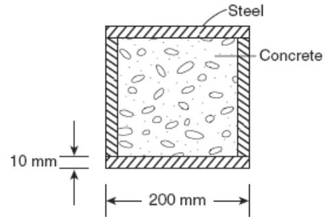
Since the composite post is subjected to compressive load, both concrete and steel tube will shorten by the same extent. Using this condition following relation between stresses in concrete and steel can be established.
