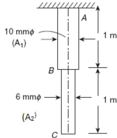
Stress at B will be due to weight of portion of the bar BC
