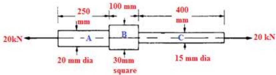
The bar consists of three sections with change in diameter. Loads are applied only at the ends. The stress and deformation in each section of the bar are computed separately. The total extension of the bar is then obtained as the sum of extensions of all the three sections. These are illustrated in the following steps.
