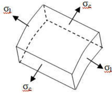
**Fig. 5 Normal stresses on the wall of thin**
