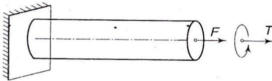
**Assignment-4:** At a point in a steel member, the state of stress shown in Figure. The tensile elastic limit is 413.7kPa. If the shearing stress at a point is 206.85kPa, when yielding starts, what is the tensile stress  $\sigma$  at the point according to maximum shearing stress theory? (**Answer: Zero**)
