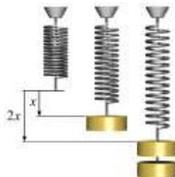
Since loads are proportional to the stresses they produce and deformations are proportional to the strains, the Hooke's law also implies that, “*stress is proportional to strain within elastic limit*”.
