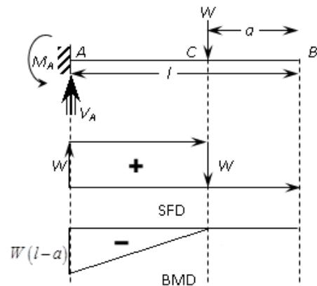
Fig. 3.33 Cantilever with Point Load
