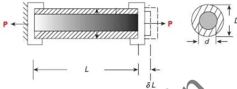
Let the extension of composite bar of length  $L$  be  $\delta L$ . Let  $E_S$  and  $E_H$  be the modulus of elasticity of solid bar and hollow tube respectively. Let  $\sigma_S$  and  $\sigma_H$  be the stresses developed in the solid bar and hollow tube respectively.
