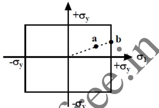
Figure- 2: Yield surface corresponding to maximum principal stress theory
