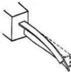
Buckling of long compression members due to *axial load*.
