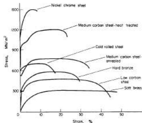
For certain materials, for example, high carbon steels and non-ferrous metals, it is not possible to detect any difference between the upper and lower yield points and in some cases yield point may not exist at all. In such cases a proof stress is used to indicate the onset of plastic strain. The 0.1% proof stress, for example, is that stress which, when removed, produces a permanent strain of 0.1% of the original gauge length as shown in the following figure.
