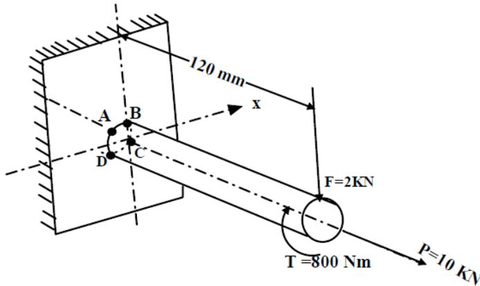
At the outset it is necessary to identify the mostly stressed element. Torsional shear stress as well as axial normal stress is the same throughout the length of the rod but the bearing stress is largest at the welded end. Now among the four corner elements on the rod, the element A is mostly loaded as shown in following figure
