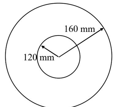
error if the maximum hoop stress is found from the equation of thin pipes?
