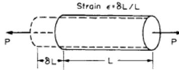
then the strain produced is defined as follows:
