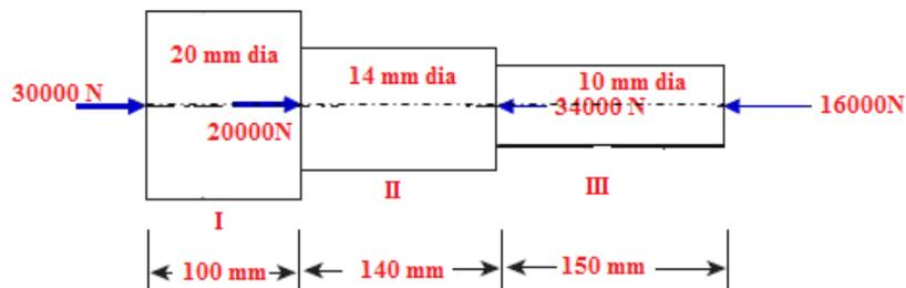
The bar is with varying cross-sections and subjected to forces at ends as well as at other interior locations. It is necessary to study the equilibrium of each portion separately and compute the change in length in each portion. The total change in length of the bar is then obtained as the sum of extensions of all the three sections as shown below.
